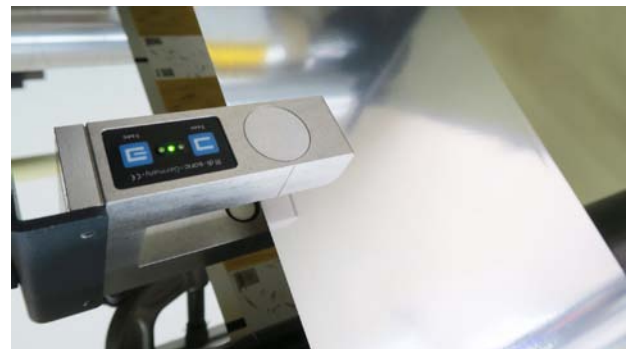
Ultrasonic Sensor DU-1S is used on reflective film
