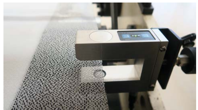
Ultrasonic Sensor DU-1S is used on mesh
